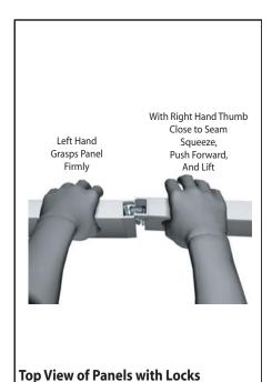
The first level of components contain pane from left to right, usually starting locks that are located at the top of the panel for extra stability and seamless connection. When disassembling panels twist top connection slightly and lift right panel upward.
