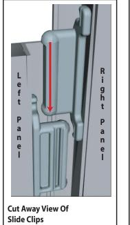
Components connect together by aligning them and sliding downward connecting clips together.
